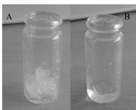
Figure 7.3. Self-healing properties of a rigid gel of 5% w/v of p(MBA-2AMPBA) and 1:1 v/v 5% w/v 125 kDa PVA. The time between the left picture and the right picture was three hours. On the left ( A ) a gel is observed that has been milled into pieces. On the right ( B ), after three hours, the same gel has completely restructured.
